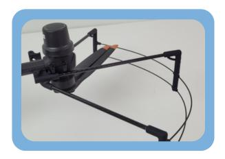
Insert propeller guard from below
