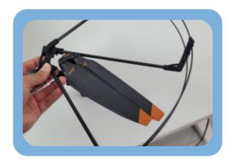
Insert propeller guard
