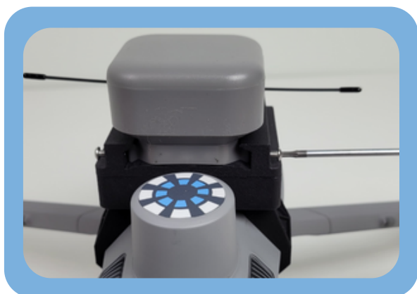
Fix the screws on the sides to hold the parachute in place.
