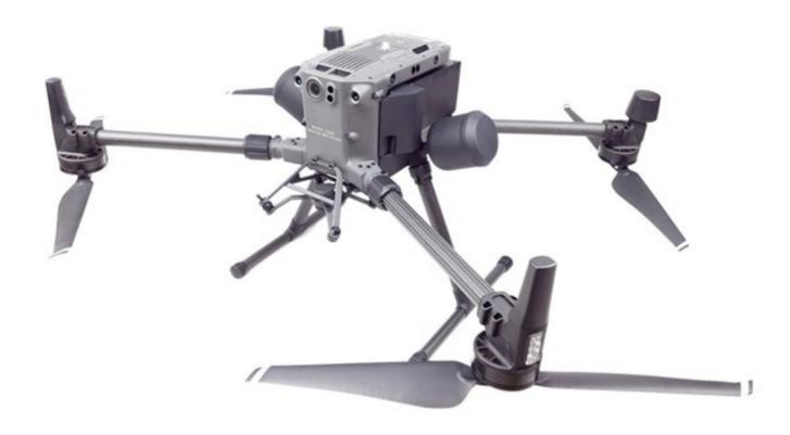
The new system for Matrice 300 RTK is safe and lightweight. It includes an ultra-fast double parachute, a circuit breaker, an alarm and a secure radio transmitter, fixed to the DJI Smart Controller Enterprise radio control system. In few seconds the parachutes can be removed, allowing the DJI Matrix 300 RTK to be folded back into its original case.
