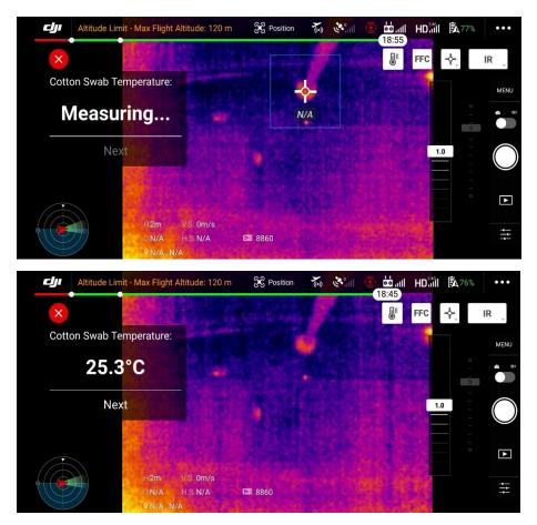
Body measurement calibration: people who are being tested should stand 2-3m away from the aircraft, with their forehead exposed. The drone operated clicks the forehead on the screen and the system will automatically obtain the forehead temperature. Click the "Next Step" button.
