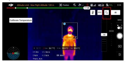
3) In point measurement mode, multiple points can be selected to ensure that the measurement position is on the forehead.
