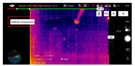
3) Click the cotton swap on the screen displaying the infrared imagery, and the system will automatically obtain the temperature of it. Click "Next Step"
