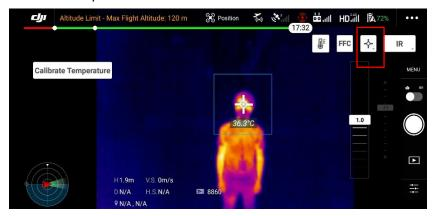
4) In point measurement mode, it is recommended to keep the distance from the subject's forehead at about 2-3 meters. In the area measurement mode, the distance can be increased appropriately.
