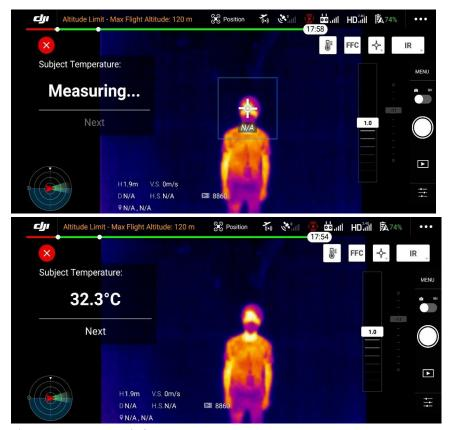
The test subject's forehead temperature should be similarly measured several times with a commonly used infrared thermometer, to be sure an accurate value is known. Input the measured value from the commonly used infrared thermometer into the DJI Pilot app as a reference, and then click the calibration button to complete the calibration.
