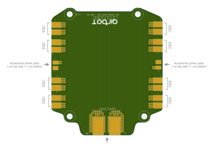
Main battery Pads 1 on top side + 1 on bottom
