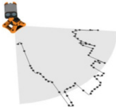
Figure 25 :: Uni-directional scanning for higher precision
