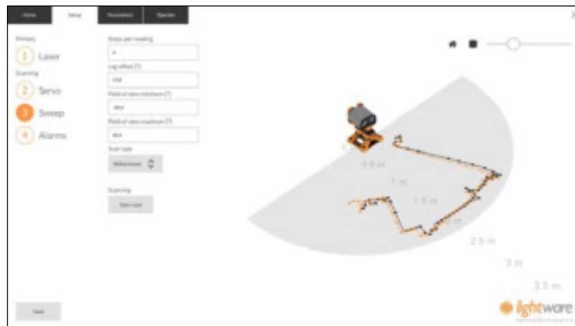
Figure 22 :: Setting up the servo's scanning characteristics
