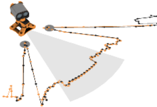
Figure 24 :: Reducing the field of view to avoid detecting the landing legs on a drone
