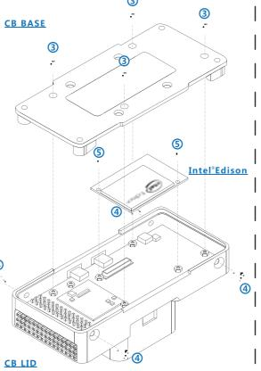
To install Intel® Edison into PIXHAWK2.1, you need to open the bottom cover of Carrier Board. Detailed procedures are as follows:
